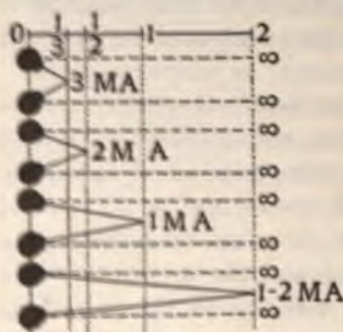
FIG. 175.—Diagram Illustrating the Unit of Convergence, the Meter Angle.
